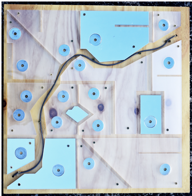
Figure 4: Top view of the Lost Oscillations user interface, showing electrodes placed throughout a map-like representation of the city center of Christchurch, New Zealand.
