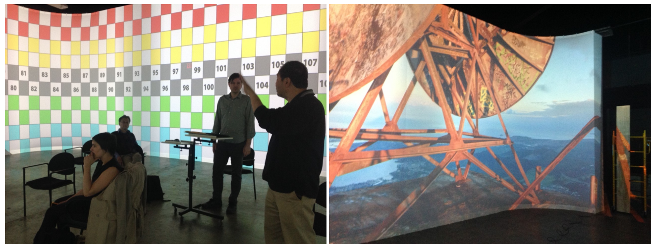
Figure 2: CRAIVE-Lab Panorama Screen. Left: Pixelwix calibration software. Right: Smooth corner solution of the CRAIVE screen.
