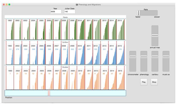
Figure 1: GUI allows control of playback start, pause, stop, volume balances, position within the dataset, and rate of iteration.
