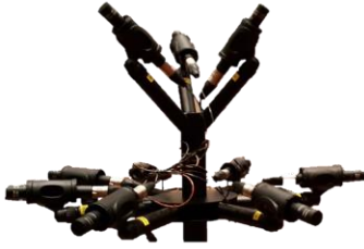
Figure 7: Picture of an implemented 10-channel microphone.
